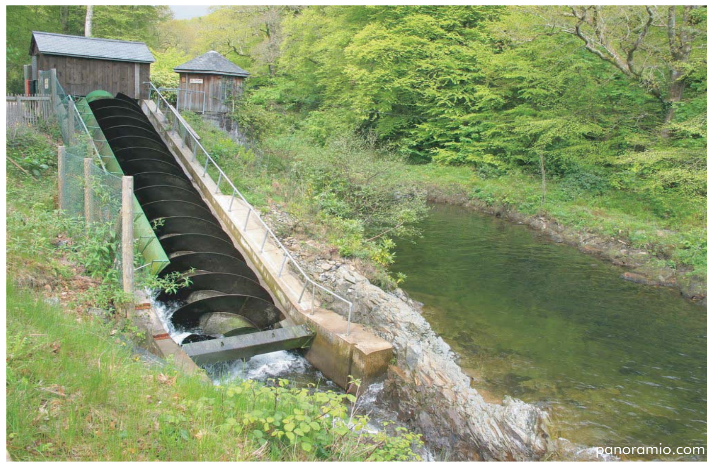
Archimedes Screw- a machine used to generate electricity from falling water
